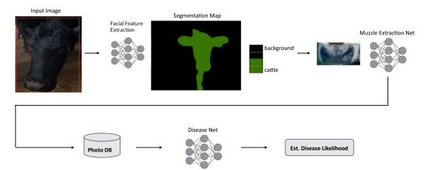
**Figure 2** Pipeline overview of the technology. Every pixel of the image is classified as either pertaining to the individual cattle or not. Machine learning extracts facial features so the computer would know what is background and what is cattle. The system ends up knowing exactly which pixels belong to a particular animal. **A** bounding box is drawn around the pertinent part of the image and cropped out. This both improves model accuracy and reduces storage and processing costs.
